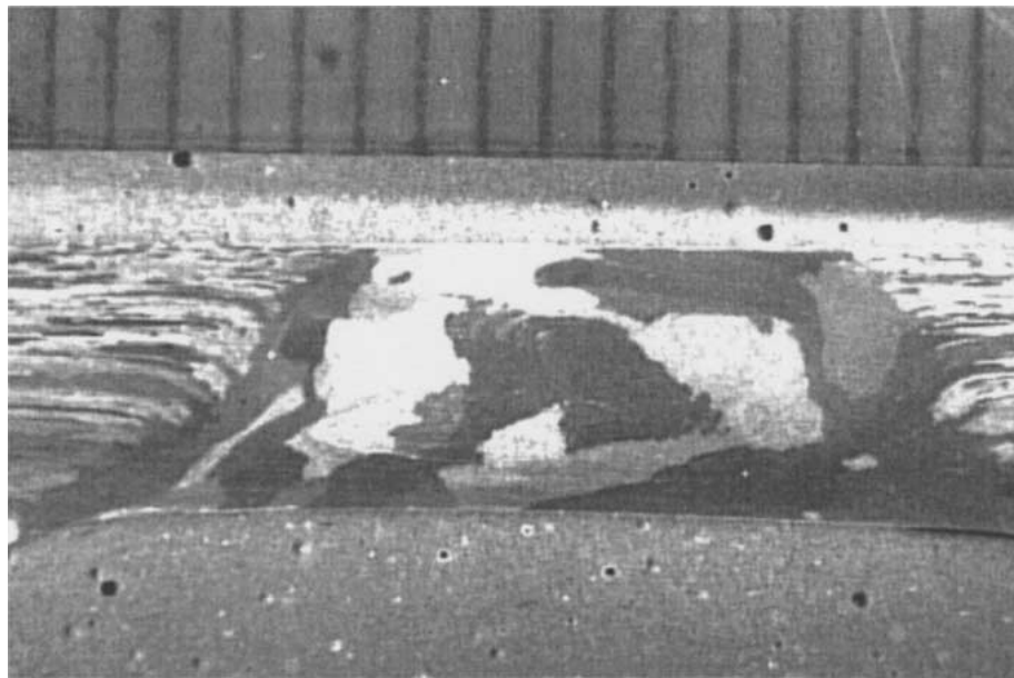
Figure 3 Post weld heat treated sample (540°C, 1 hour + 175°C for 8 hours) showing coarse grains in the weld region.
